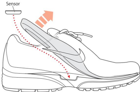
You can leave the sensor in your shoe when you aren't working out, but if you plan to wear your shoes for a long time without working out, replace the sensor with the foam insert to save battery life.
